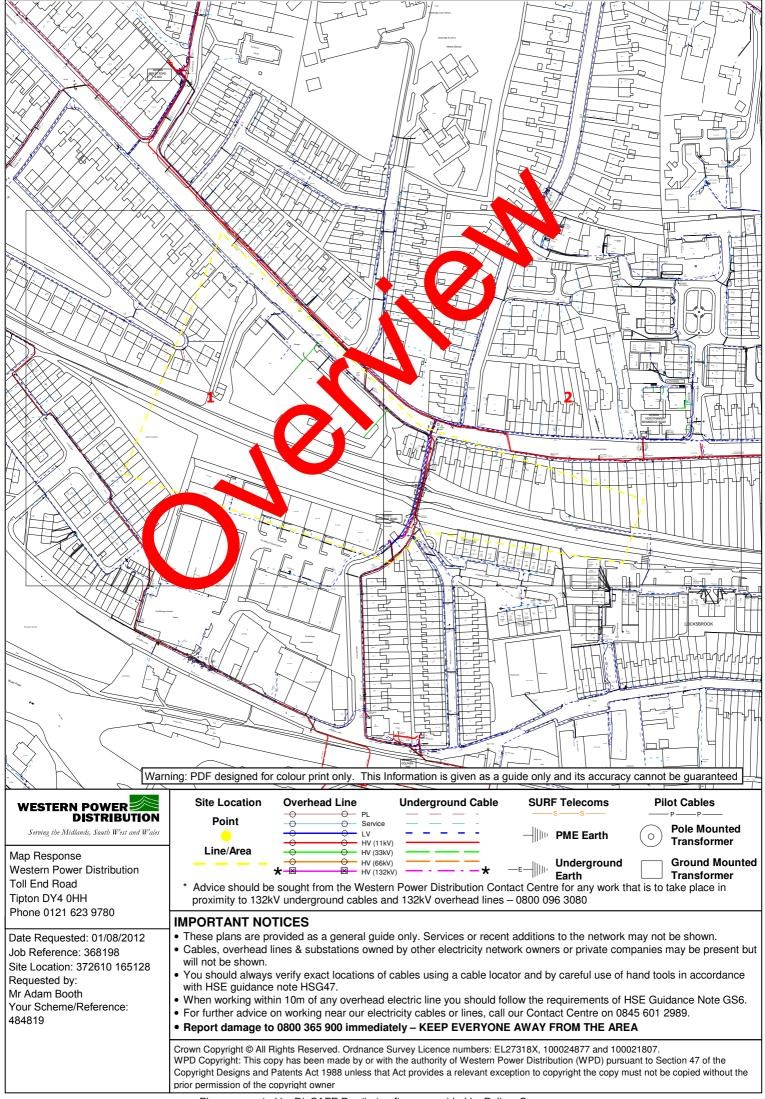
Plans generated by DigSAFE Pro (tm) software provided by PelicanCorp
