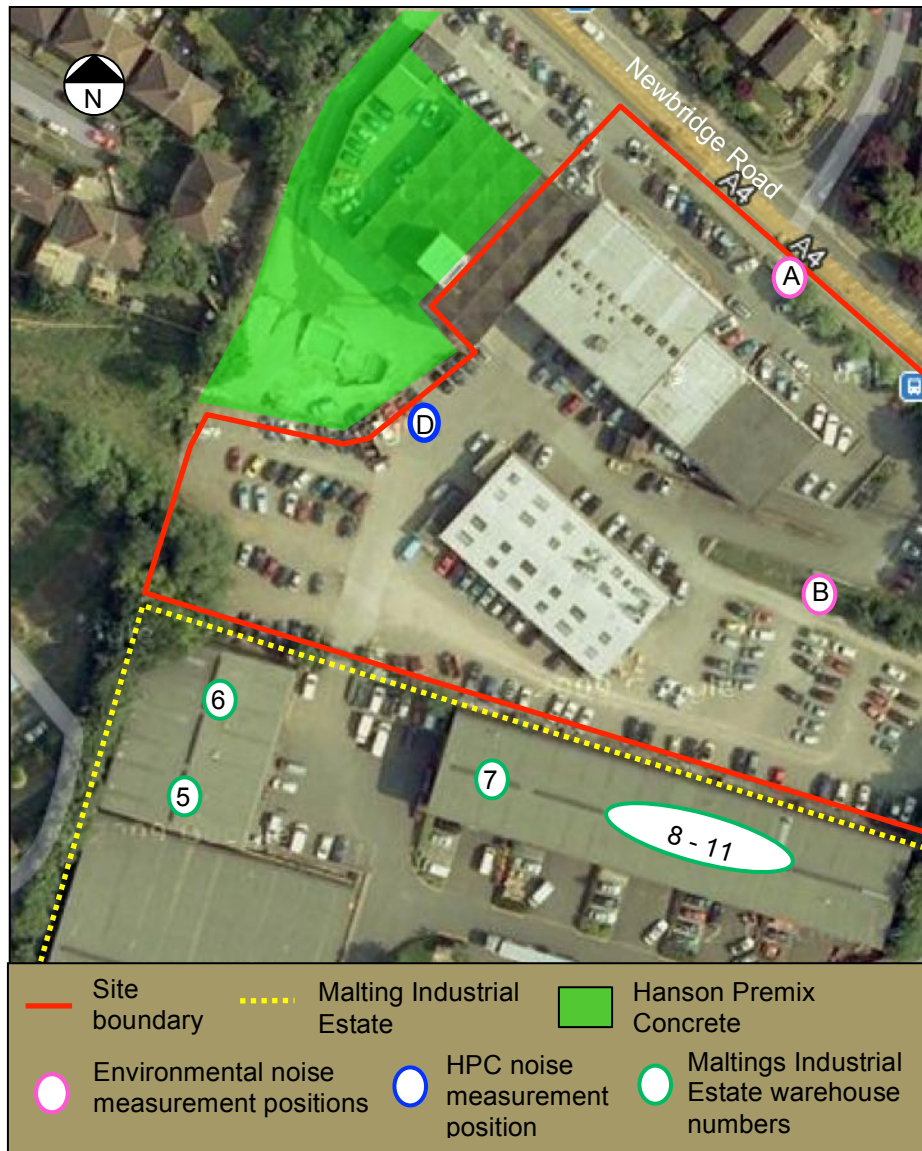
Figure 1. Aerial view (source: www.google.com) showing proposed site, existing industrial developments and noise measurement positions
